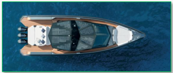
WALLY Wallytender with photovoltaic panels*
