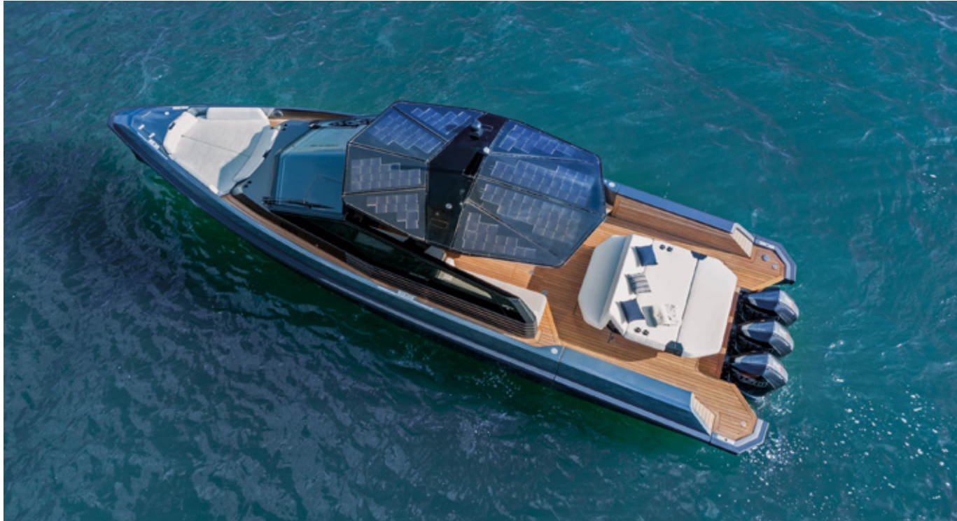
wallytender43X with solar panels on roof
