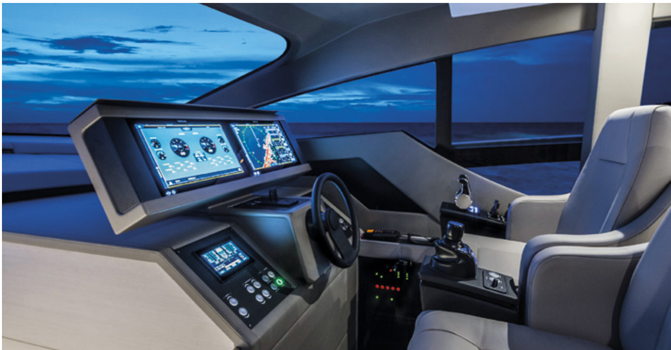
The Joystick Yacht Control of the Pershing 7X'
